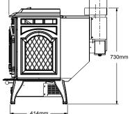
Figure 20.8 - Side View with Top Vent Adapter
